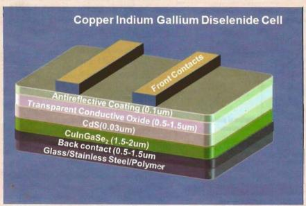
(Above) Construction differences for crystalline and amorphous silicon cells and for CIGS and CdTe cells become evident from their cross sections.
